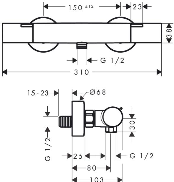
**Ecostat Fine****Mitigeur thermostatique douche C3**Finition: Chromé    Numéro d'article: **13326000**
